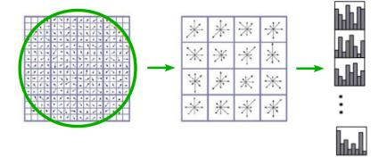
Figure 2.12: Illustration of SIFT descriptor formulation.
