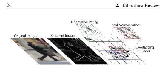
Figure 2.13: Illustration of HOG descriptor formulation.
