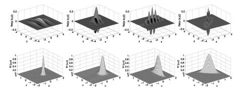
Figure 3.2: Example of a 2D Gabor filter in the spatial and frequency domain.
