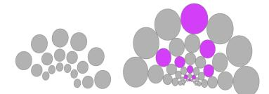
**Figure 3.6:** Examples of a fixed size traditional bank of Gabor filters and a bank used in a novel randomized GMM approach. Left: The traditional approach – a small Gabor filter bank from where responses of all filters form the feature vector (e.g., [179, 75, 191, 87]); Right: a large bank from where the part characteristic frequencies are selected by the random optimization process. [141]
