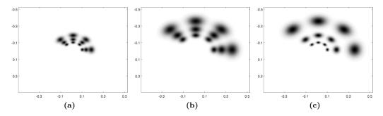
**Figure 3.4:** Examples of a multiresolution set of Gabor filters in the frequency domain: (a) M = 4 orientations and N = 3 frequencies, (b) the base frequency  $f_{max}$  increased, (c) the frequency scaling factor k increased.
