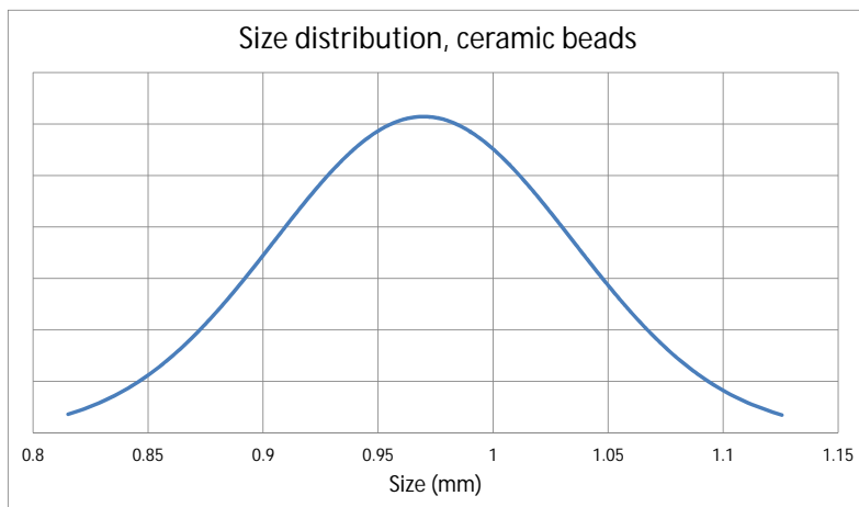
Figure 6.3. Normal distribution of the ceramic bead size in the COOLOCE experiments (image analysis).
