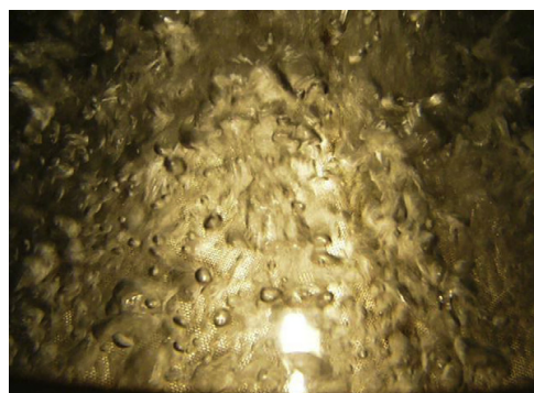
Fig. 5. Steam bubbles near the surface of the conical particle bed.
