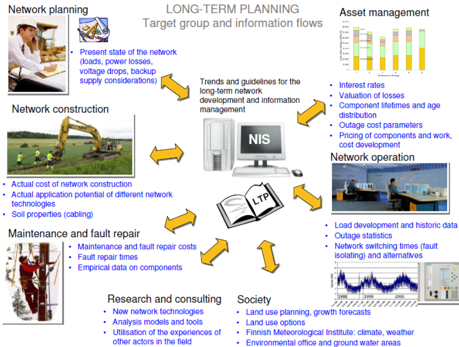
Figure 1.1. Long-term planning of electricity distribution (Lassila, 2009).
