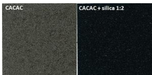
Figure 22 Scanned images in from sample from the 100% black ink areas printed on CACAC surfaces with and without silica.
