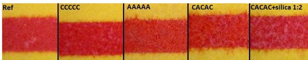
Figure 20 Photomicrographs of the lateral bleeding of red ink.
