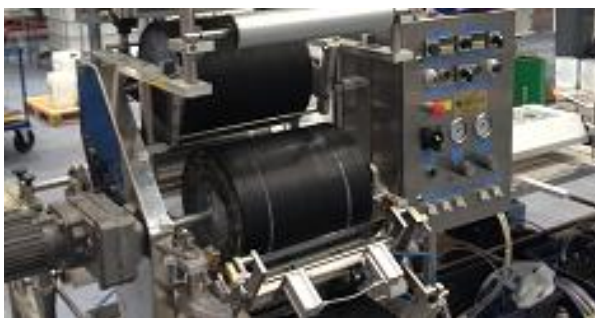
Figure 5 Pilot coater (DT Laboratory Coater, DT Paper Sciences, Turku, Finland).
