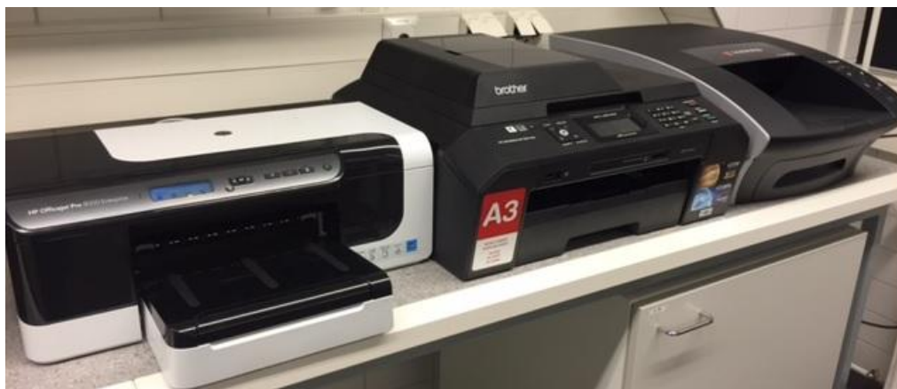
Figure 6 (Left) HP Officejet Pro 8000 Enterprise printer, printer 1 , (middle) Brother MFC-J5910DW printer, printer 2 , and (right) Memjet, Lomond Evojet Office printer, printer 3 .
