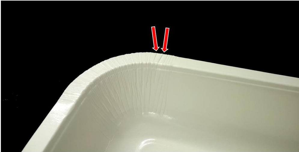
Figure 20: Unacceptable creases in the tray flange. The creases have not been formed adequately, leaving a gap between the flat areas surrounding the crease.
