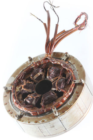
Figure 1: Six-slot two-pole prototype for a small high-speed PMSM
