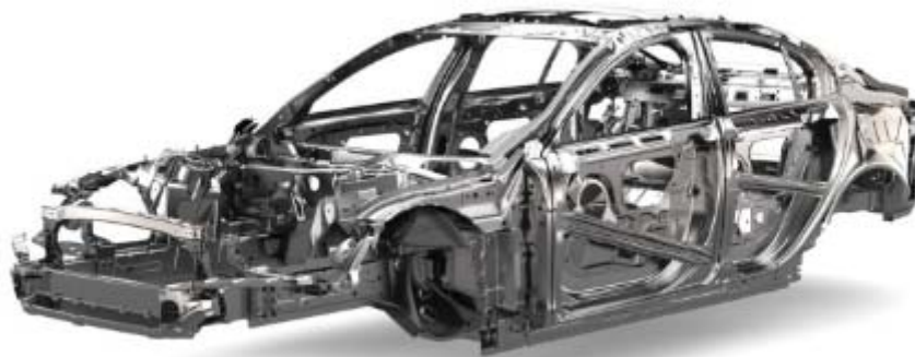
Figure 7. Jaguar XE monocoque chassis frame (Strauss, 2013).
