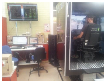
FIGURE 9. VIRTUAL SIMULATOR CABIN ENABLES INTERACTIVE SIMULATION WITH A HUMAN OPERATOR.
