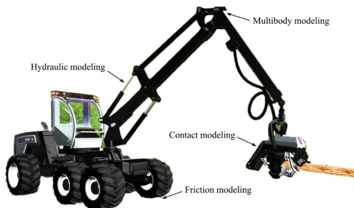
Figure 2.1: Modeling tasks involved in the real-time simulation (adapted with permission from Mevea Ltd.)
