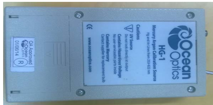
Figure 18. Ocean Optics HG-1 Mercury Argon Calibration Source.
