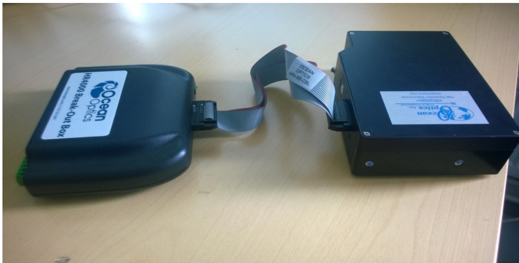
Figure 5. Spectrometer connected to Break-out Box using serial cable HR4-BB-CBL.
