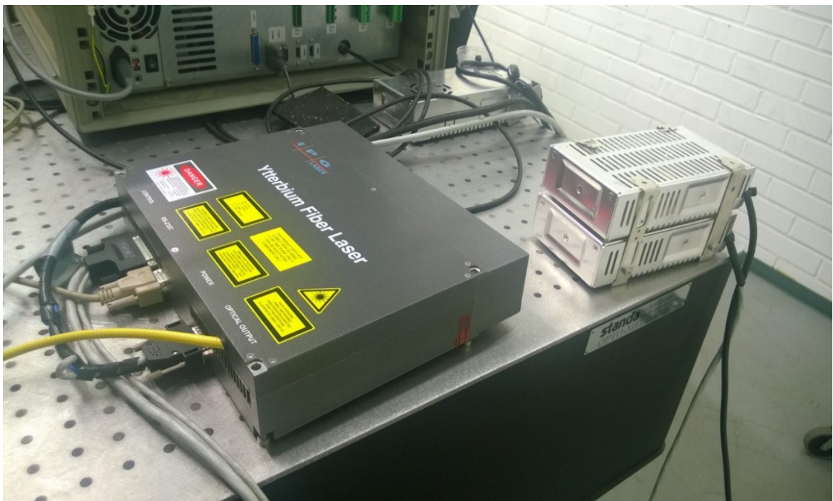
Figure 19. IPG 20 W ytterbium pulsed fiber laser and its power sources.
