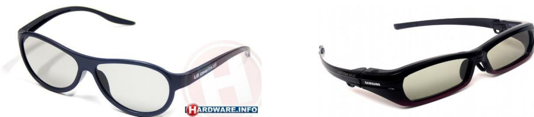
Figure 2.14. Passive (left) and active (right) shutter glasses (Ballegoie, 2012; Campbell, 2011).
