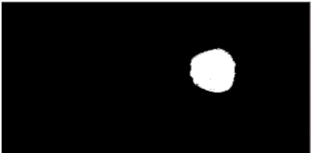
Figure 2.22. Image after finding the exact color range in H, S, V (Fernando, 2013).
