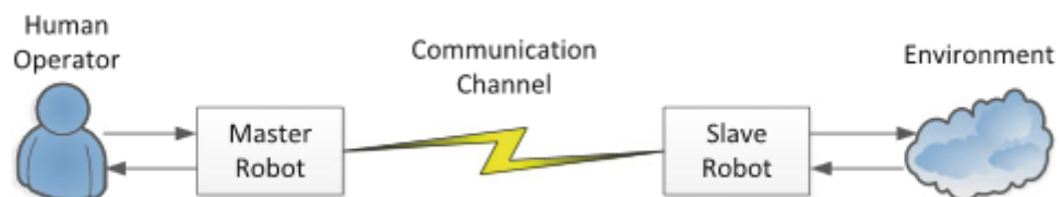
Figure 1.1. Scheme of tele-operated robot (Li & Su, 2015).
