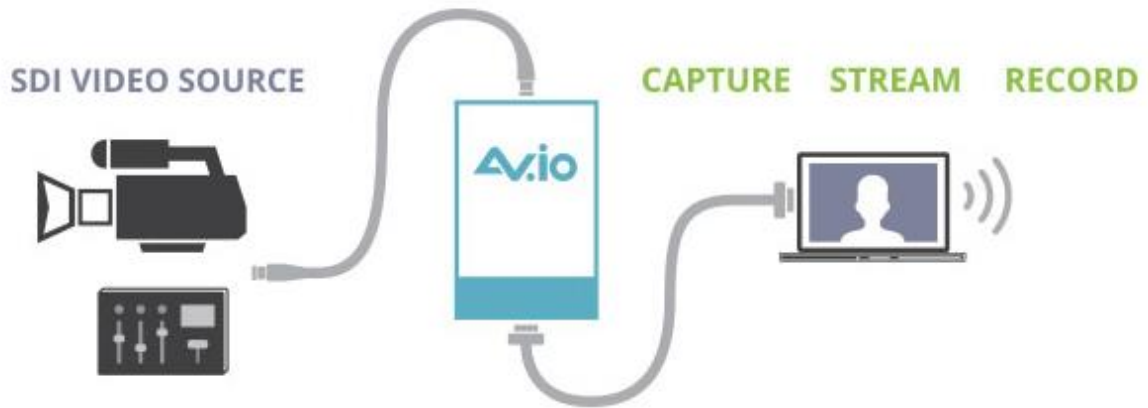
Figure 3.9. Scheme of frame grabber's operation (Epiphan Video, 2016).
