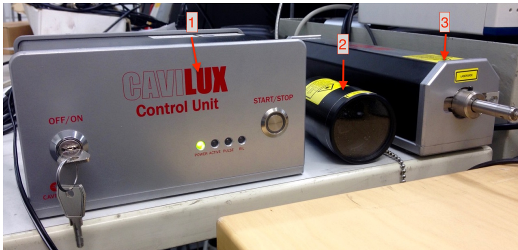
Figure 8. CAVILUX HF illumination system (1. Controller, 2. Laser lens, 3. Laser unit).
