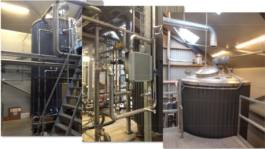
Figure 4: A biological methanation reactor used in the Foulum project, Denmark [20, p. 16].
