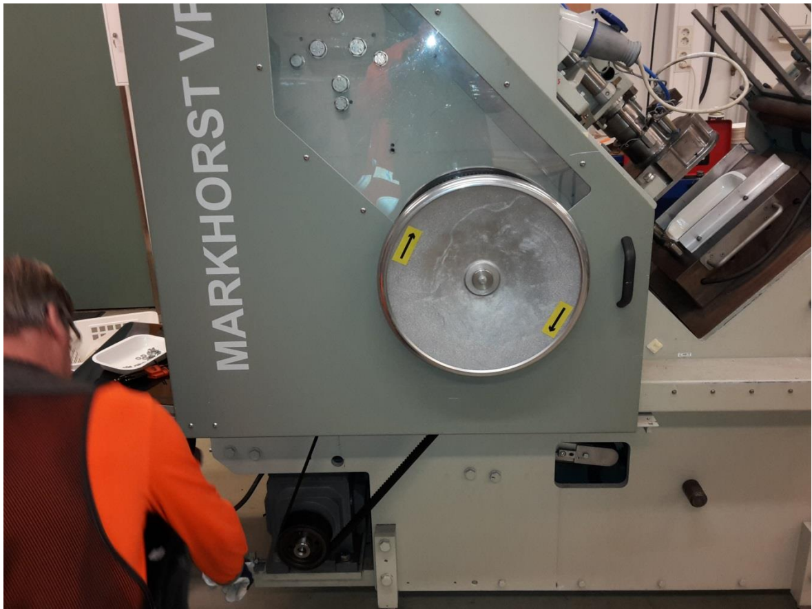
Figure 31. Main drive shaft belt change.
