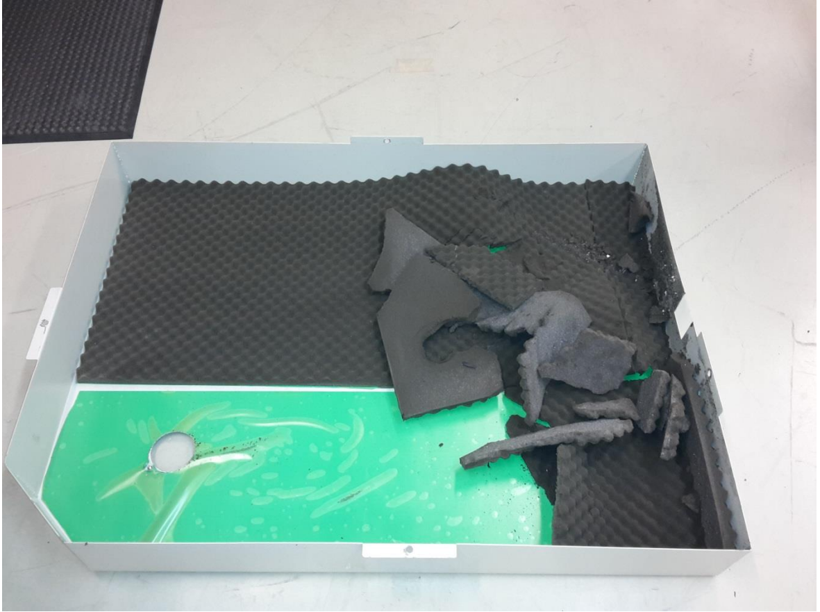
Figure 30. Brittle sound dampening foam.
