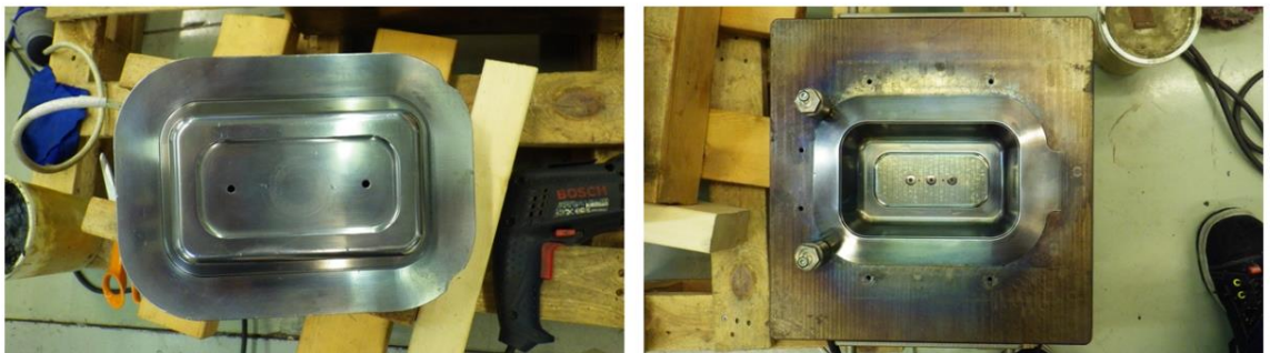
Figure 40. Mould tools before and after polishing.
