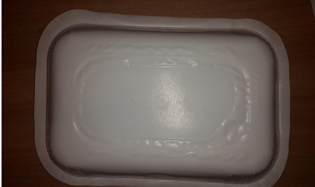
Figure 62. Delamination of layers due to steam explosion.
