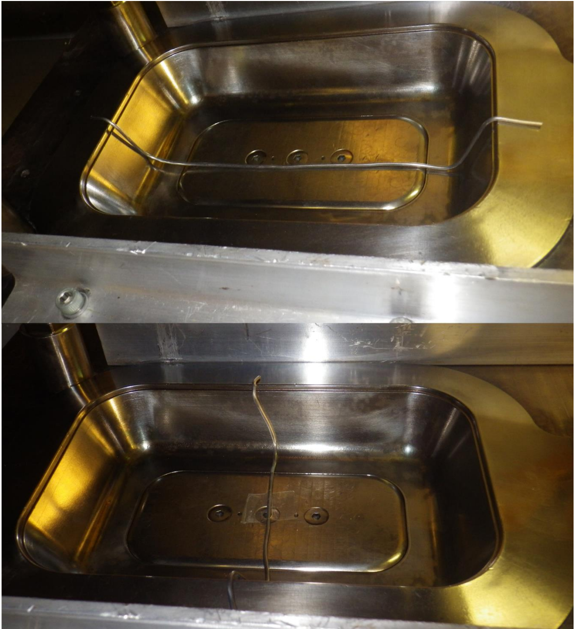
Figure 33. Tin wire placement used for measuring alignment.
