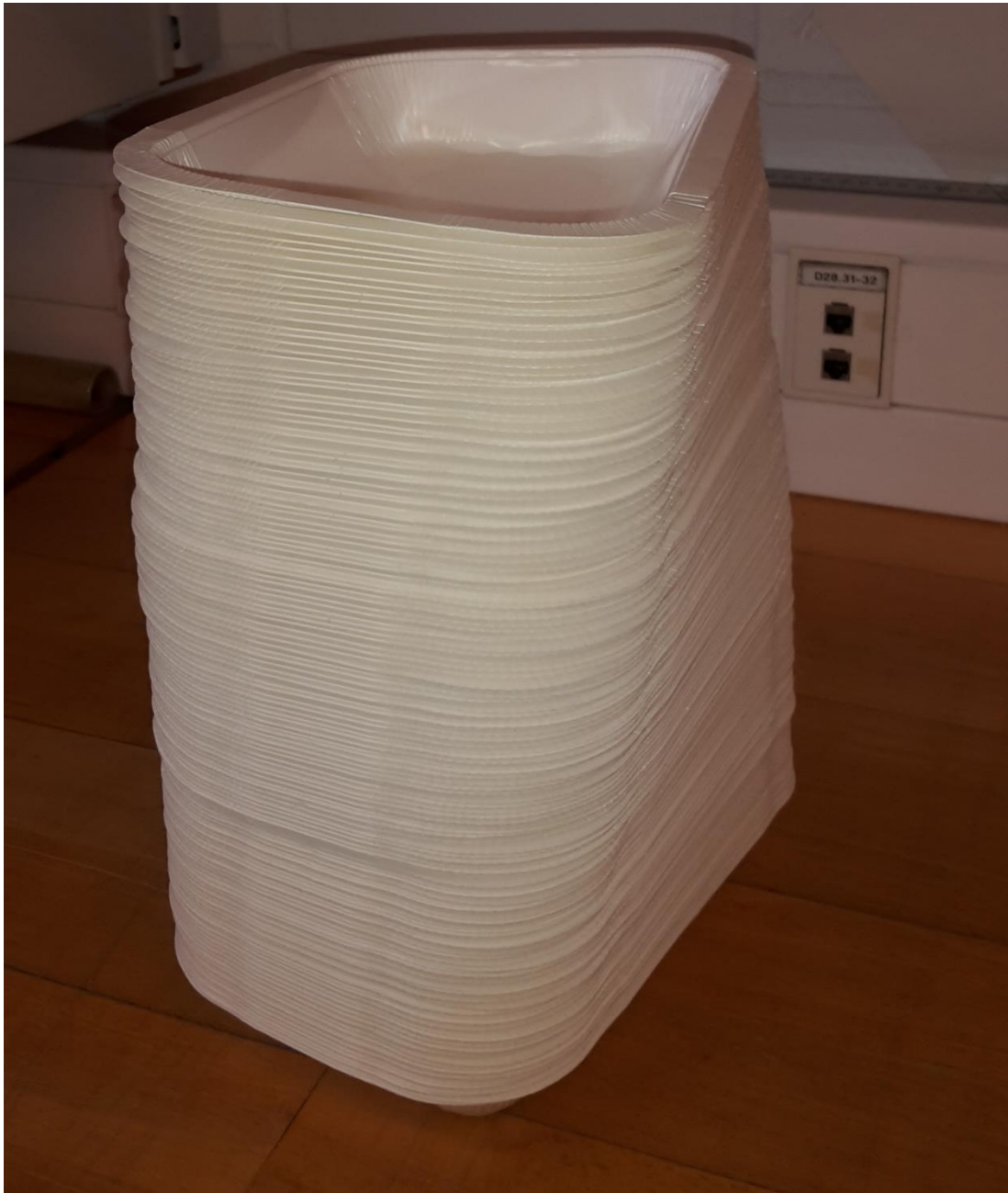
Figure 34. Twisted tray stack indicates improper tool alignment.
