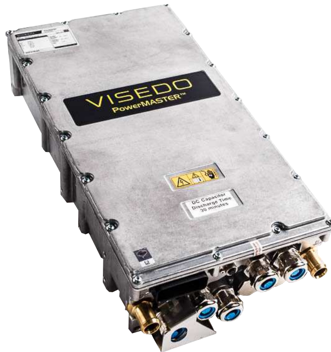
Figure 4. Visedo Oy's PowerMASTER M-frame. The device has connections for DC-link, three phase AC-voltage connection, cooling liquid connections, AMPSEAL 35-pin connector and a maintenance port.
