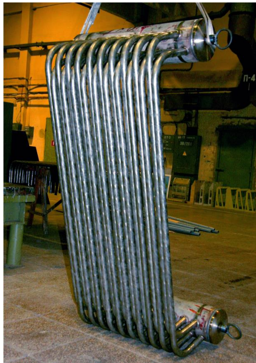
Figure 21. General view of the model of the heat exchanger-condenser in the KMS facility [34].
