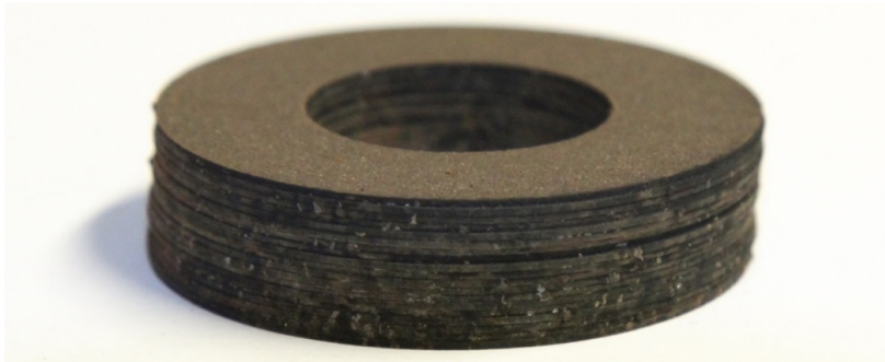
Figure 3.8 Lamination sample glued with VOLTATEX E 1175 W TM (Axalta, 2016) after the aging test, 500 hours at 160 °C temperature
