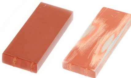
Figure 7. Coated sample D 2 (left) and artificially damaged sample D 2 (right).
