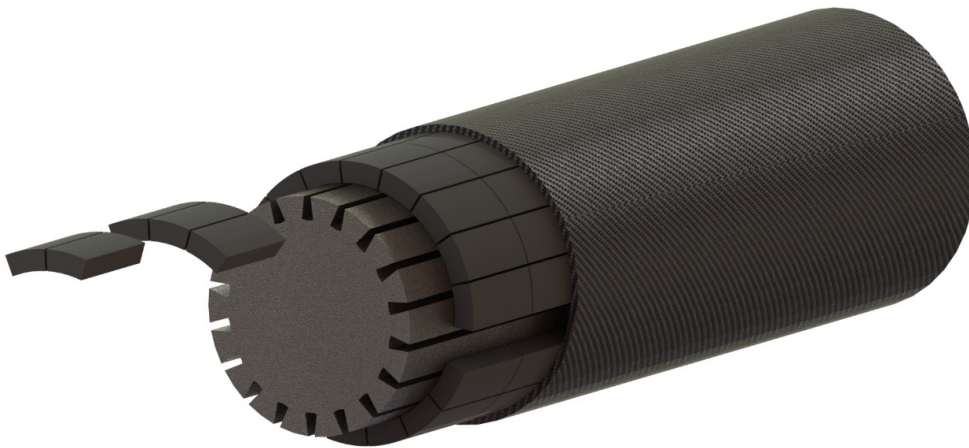
Figure 1.5 Rotor model of the rotor-surface-magnet HS PMSG. Slots under the magnets are used for the rotor cooling
