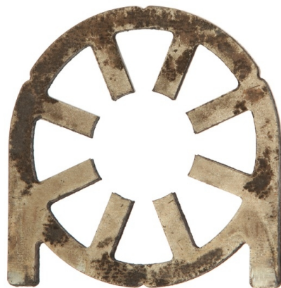
Figure 3.7 Lamination sample glued with Suralac 9000™ (Cogent, 2016) after the aging test, 500 hours at 160 °C temperature
