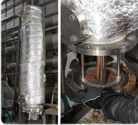
Figure 6. Photo of the test column (left) and assembling of the bottom part (right).
