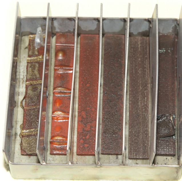
Figure 3.5 Magnetic wedge samples after the aging test, 300 hours at 150 °C temperature
