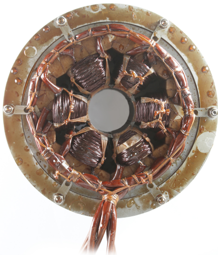
Fig. 4. 11 kW prototype for a small high-speed PMSM
