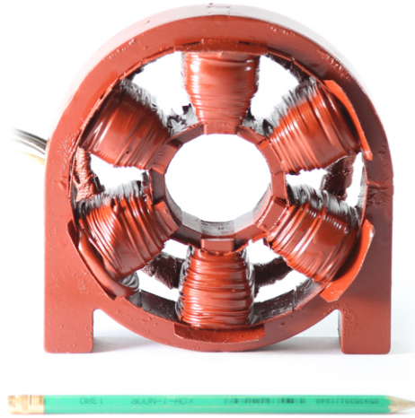
Fig. 5. 3.5 kW High-Speed Permanent Magnet Synchronous Machine stator
