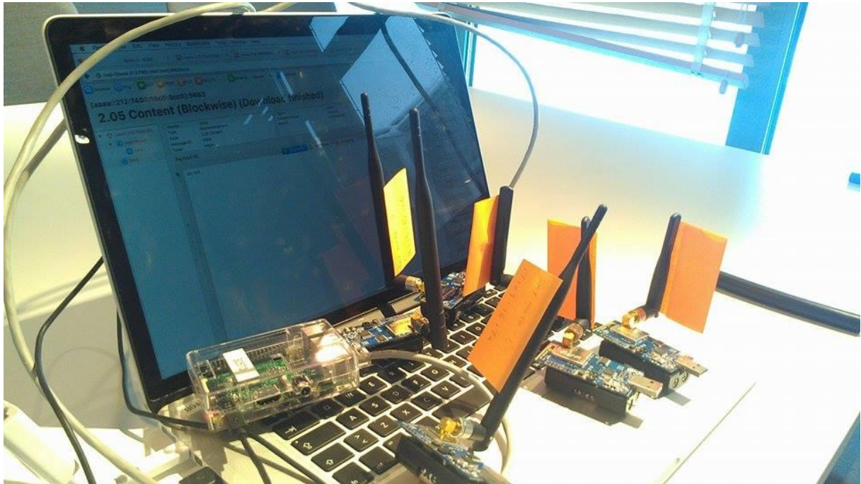
Figure 35 – RPi running 6LBR, connected over USB to the slip radio and via Ethernet to a development PC and the various sensors running CoAP servers
