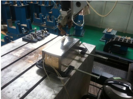
Figure 4.28 Experimental setup to record the heat cycle
