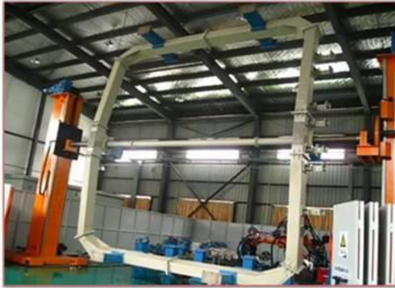
Figure 3.14 Overview of actual welding tilter
