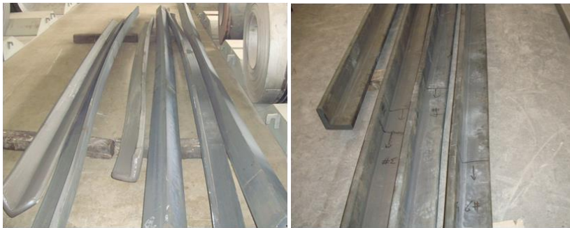
Figure 2.9 Extruded L-shaped steel (before and after straightening)
