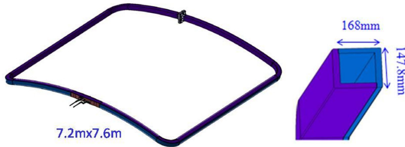
Figure 1.4 SCC case structure
