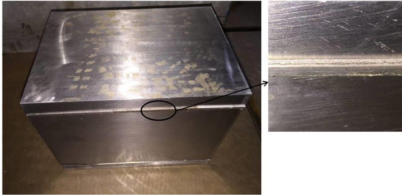
Figure 4.20 Laser welding results of scheme 1 for backing strip
