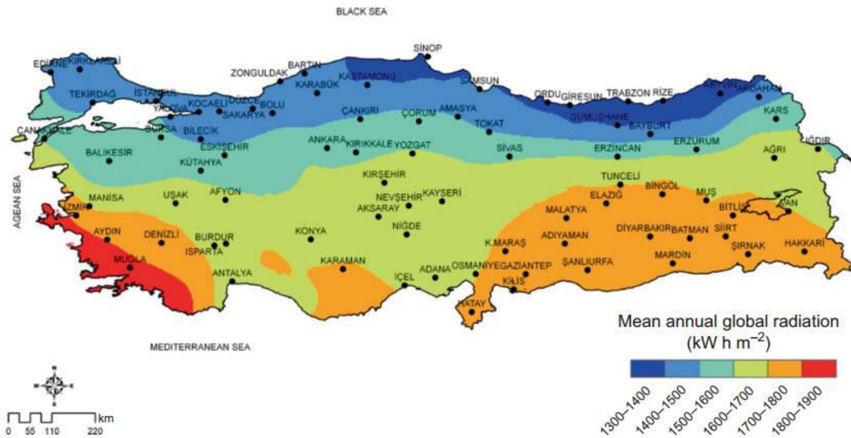
Figure 25. Average of 22 years of Turkey's annual global solar irradiation distributed geographically (Aksoy, 2011).
