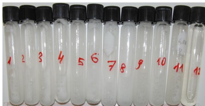
Figure 24 – Test-tubes with pH changing from 0 to 14. Liquid volume: 10 ml. BP amount: 0.2 g. pH in #9 is 11 and increases up to 14 in-#12.
