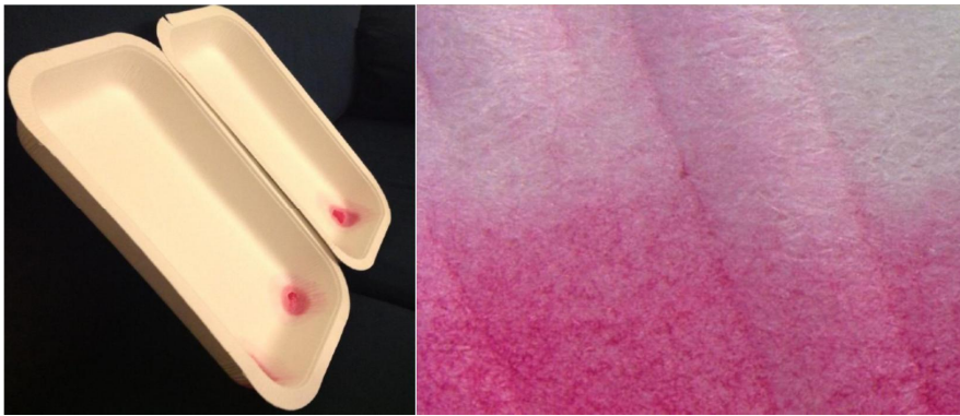
Figure 6.2 Positioning of trays in OGR testing (left) and a close-up of an oil stain at a tray corner.
