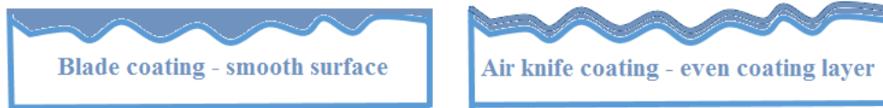
Figure 2.2 The difference between a blade-coated and air-knife-coated surface. Film and rod coating methods provide a compromise between an even surface and a constant thickness. (Redrawn and modified from Kimpimäki 1998)
