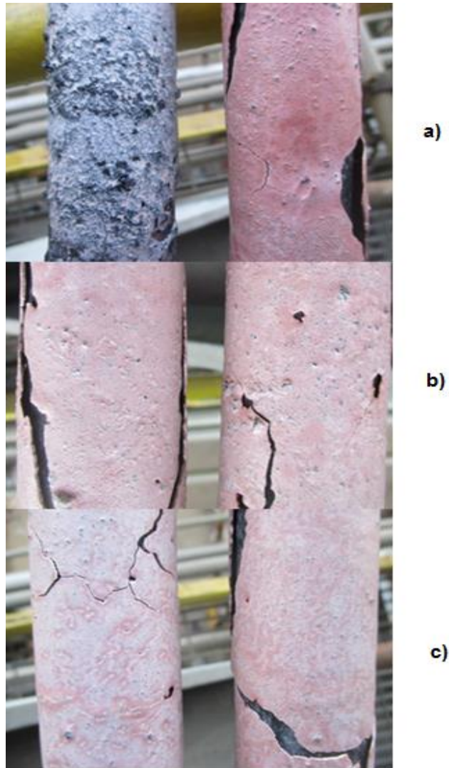
Figure 8. Smelt reduction samples of a certain recovery boiler, with boiler load of 1100 tDS/d and with different distribution of combustion air. The amount of total air and steam were maintained constant during every sampling. Grey or lighter red colour of the sample indicates the reduction efficiency degree, which is increasing from left side sample A to C. Right side sample A has a good reduction, since it contains unburned carbon, occurring as black residue on the surface of the sample. The amount of primary air fed to boiler is the lowest in case A sample, and the highest in case B. The amount of tertiary air was increased as a relation to primary and secondary air in every case. The highest tertiary air condition was in case A, and the lowest in case B. (Andritz Oy , 2015)
