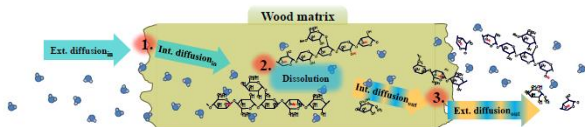
Figure 7: Simplified layout of the extraction process of hemicelluloses from wood (Krogell, 2015)
