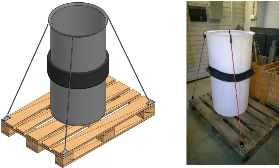
Figure 8. Palletised bending test arrangement concept (left) and realised.
