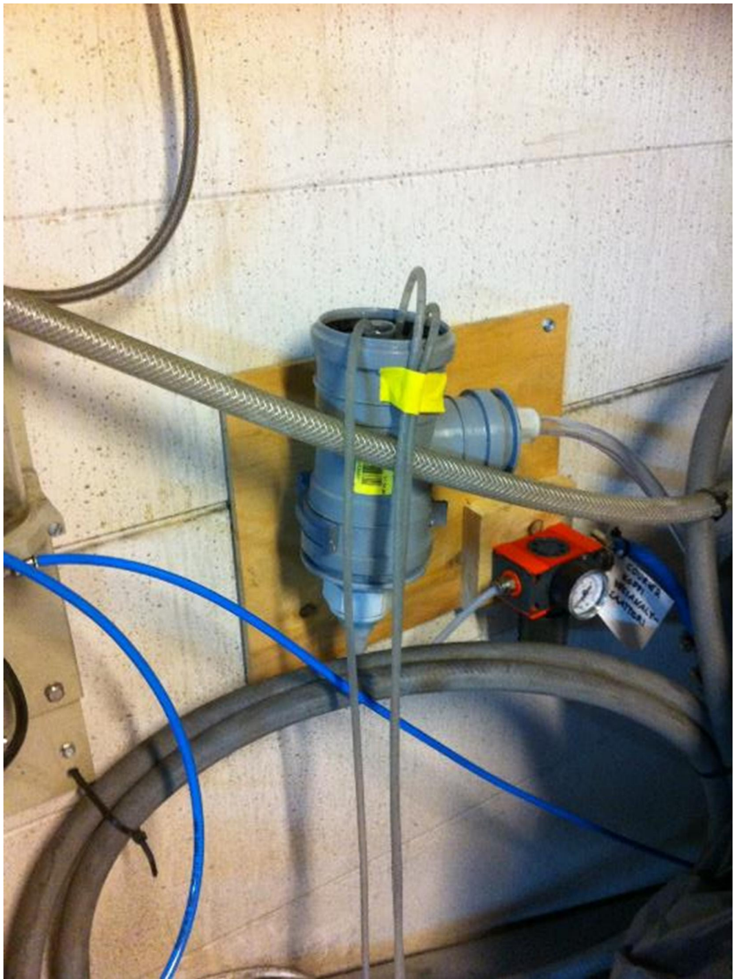
Figure 19. Process water sample basin is feed from the bottom of the basin with a constant over flow. Sample lines for the peristaltic pump are also visible the one in the middle is the feed line and two from the side are the circulation lines.
