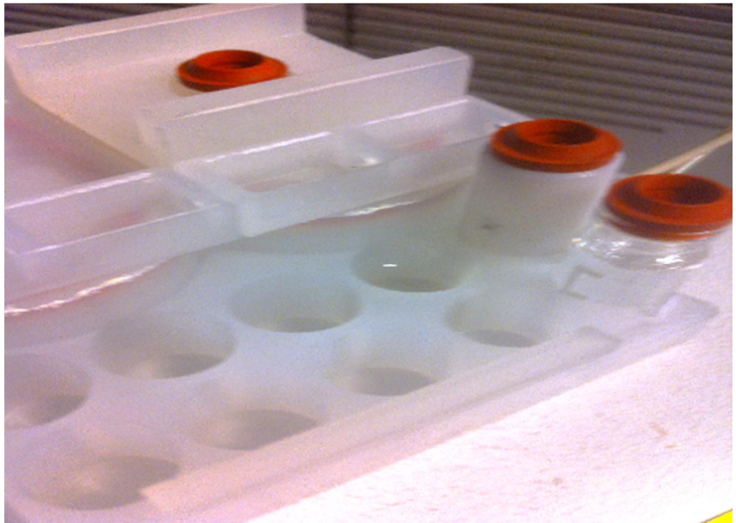
Figure 59 After the vial has overflown current leakages are likely to happen.
