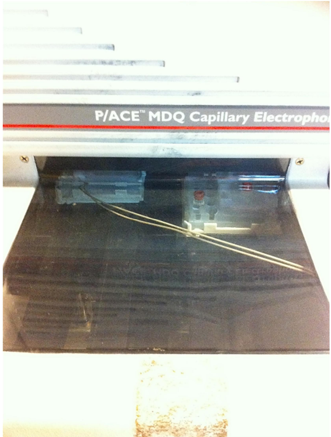
Figure 14. Sample is circulated into the sample container trough the pipes.
