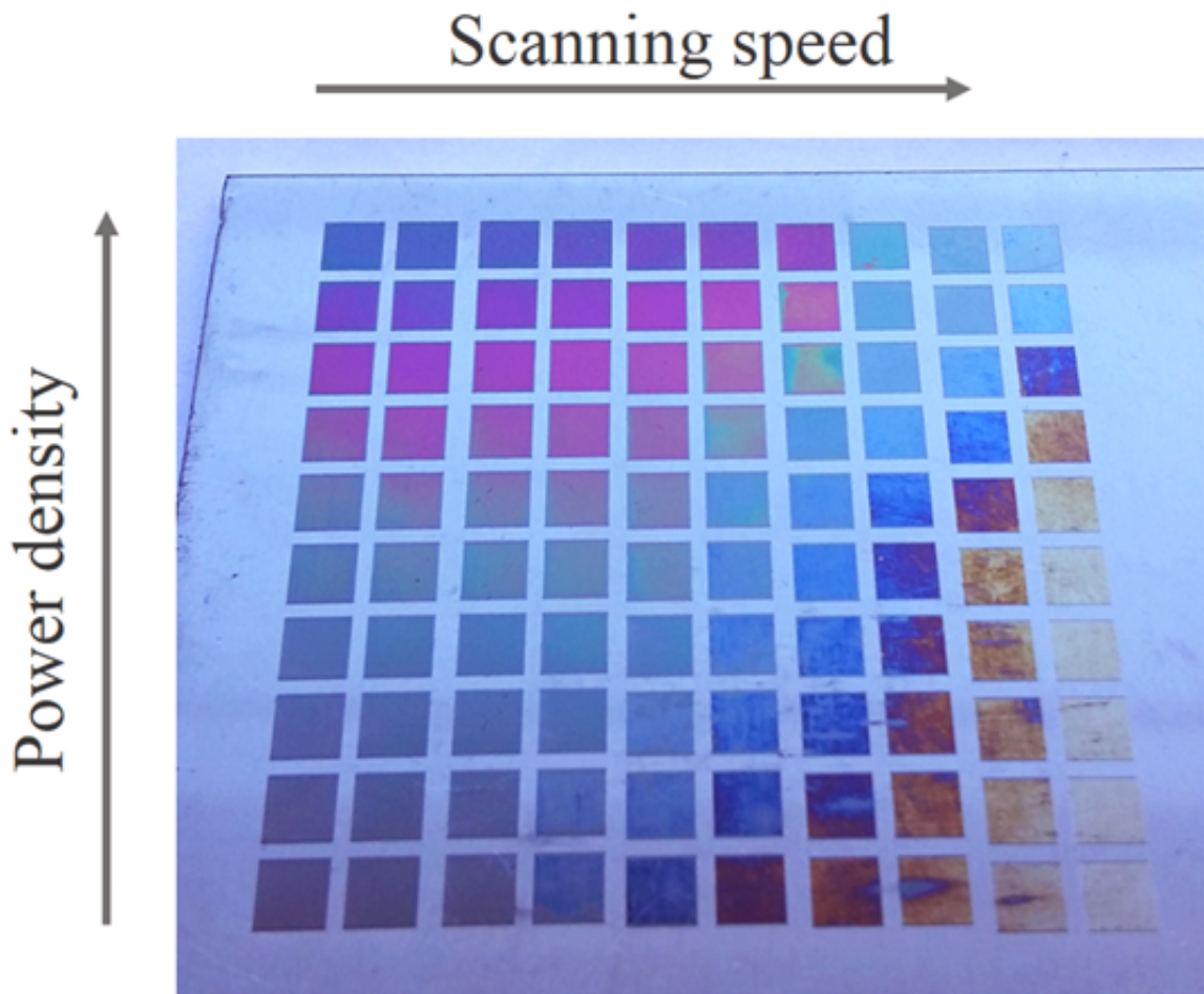
Figure 14. The dependence of produced color on the power densities I_0 = 8 \cdot 10^7 \div 1.6 \cdot 10^8 W/cm^2 from up to bottom; scanning speed 450 \div 900 mm/s , f = 60 kHz, \tau = 100 ns, H = 0.01 mm.
