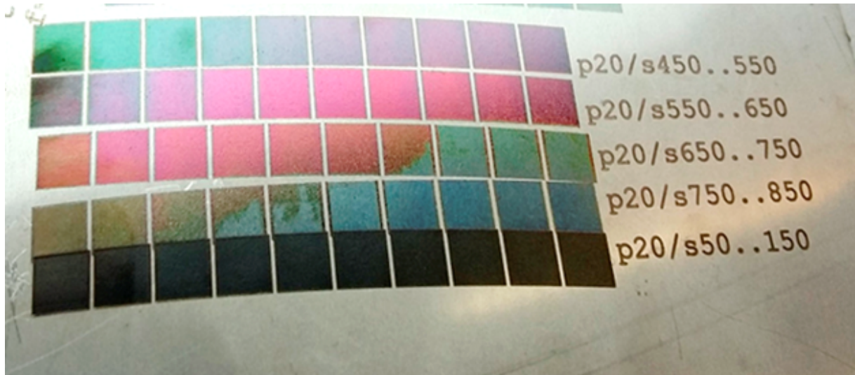
Figure 15. The dependence of produced color on the scanning speed. I_0 = 1.6 \cdot 10^8 \text{ W/cm}^2 ; f=60\text{kHz} ; \tau=100\text{ns} ; H=0.01 \text{ mm} ; scanning speed 450 \div 850 \text{ mm/s} (line 1 to 4), 50 \div 150 \text{ mm/s} (line 5) from left to right.
