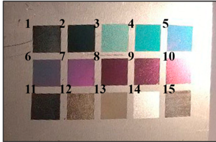
Figure 30. The color palette after 24hs exposure in the environmental chamber at T = -40\text{ }^{\circ}\text{C} with humidity of 90%.
