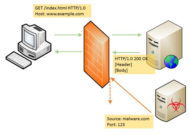
**Figure 3.** Hardware firewall blocks unknown packets and lets allowed packets through.
