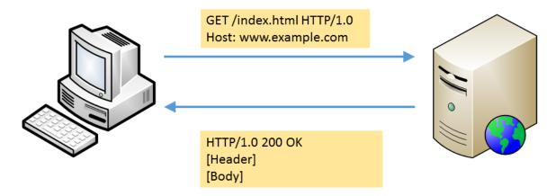
**Figure 1.** An HTTP (Hyper-Text Transfer Protocol) request-response where a browser requests an HTML file from a webserver.
