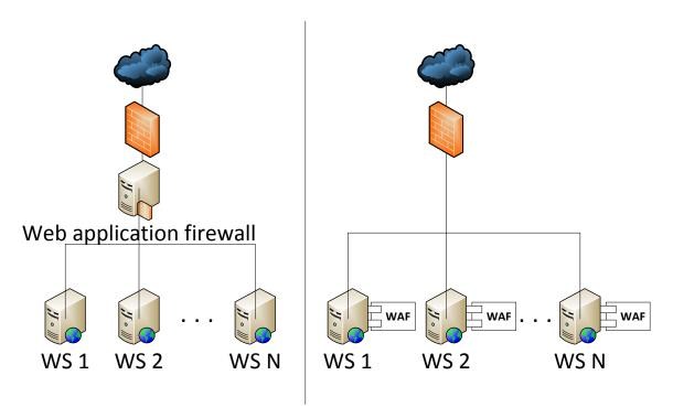
Figure 4. Reverse proxy on the left and web server (WS) embedded WAF on the right.
