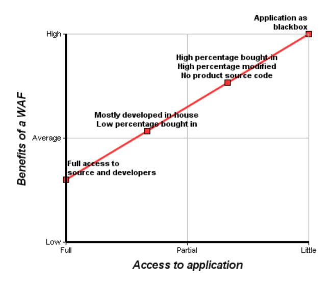
**Figure 5.** Benefits of a WAF for different levels of access to an application [4].
