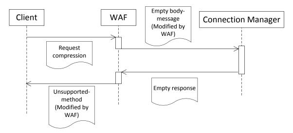
**Figure 11.** WAF suppresses the compression request of the client.
