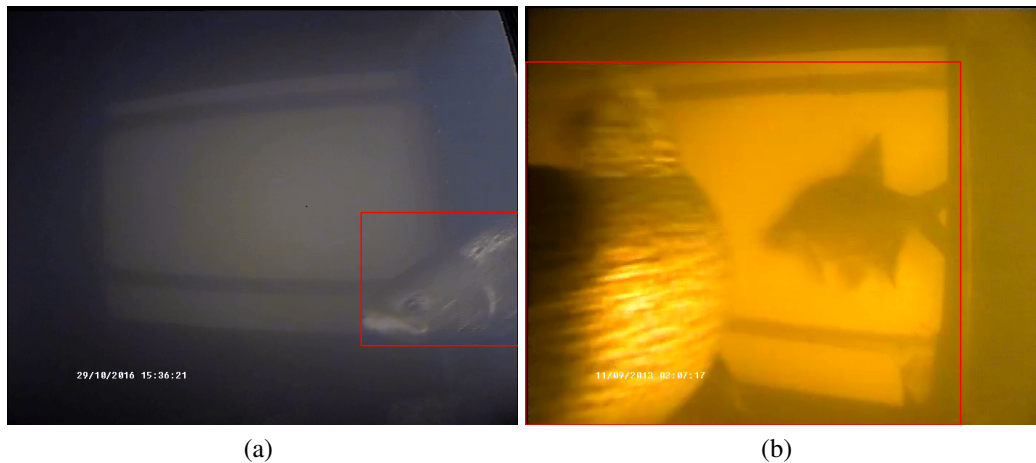
Figure 22. Challenges in size estimation: (a) Only a part of the fish is captured; (b) Incorrect detection.
