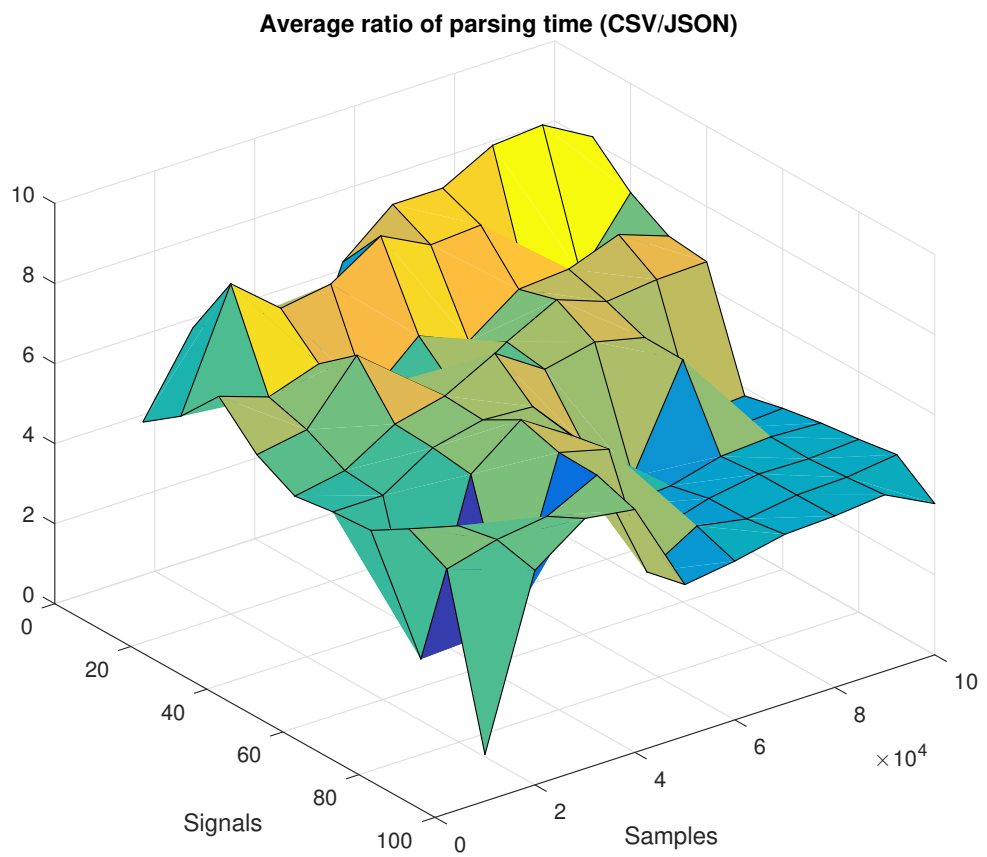
Figure 12. The ratio of CSV parsing time against JSON parsing time. From this figure, it can clearly be seen that parsing data from CSV format takes on average at least four times the time it takes to parse similar data from JSON data.
