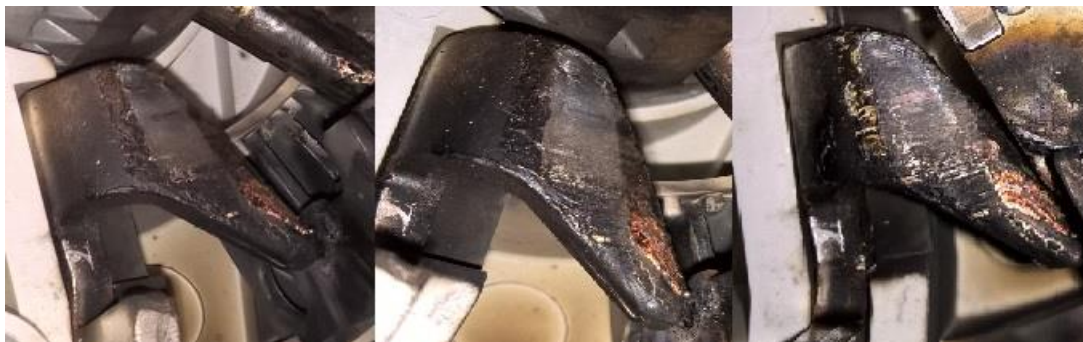
Figure 3.2 Carbonisation and polymerization of a the lubricant on the contact surface after 200 operations
