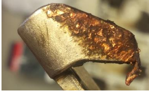
Figure 3.19 The fixed contact of OT400. Black areas showing burnt lubricant trapped in degraded contact surface.
