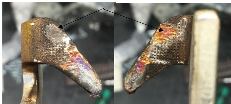
Figure 6.2 Black arrows showing main area of contact of the modified contact sample after 1000 electrical operations.
