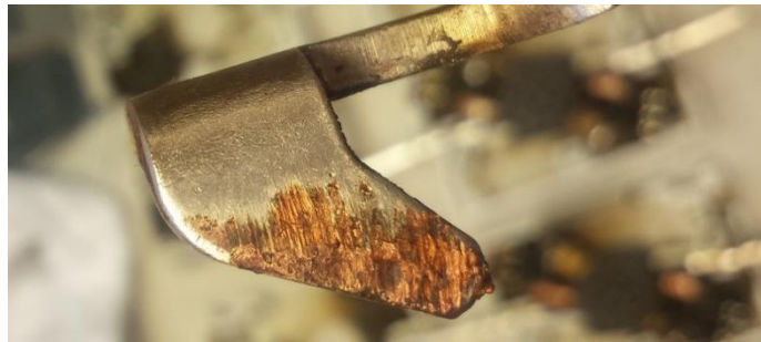
Figure 3.11 Eroded contact of OT400 after 2000 operations.
