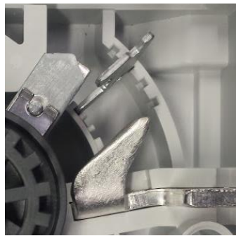
Figure 5.4 Arcing plates in samples c.
