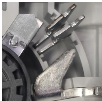
Figure 5.2 Arcing plates in sample a.
