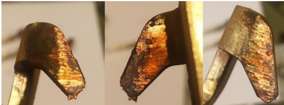
Figure 3.20 Contact wearing of OT400 with no-grease 2000 operations.
