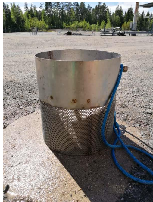
Figure 3.2. Pellet sampling device, mesh size 0,43 mm.
