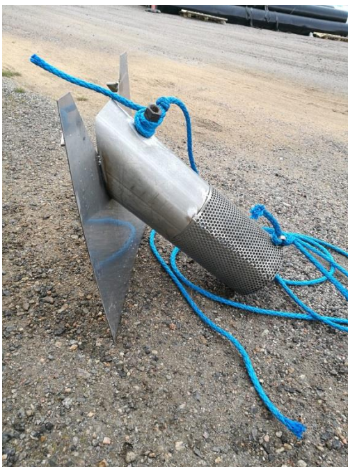
Figure 3.1. Pellet sampling device, mesh size 0,43 mm.
