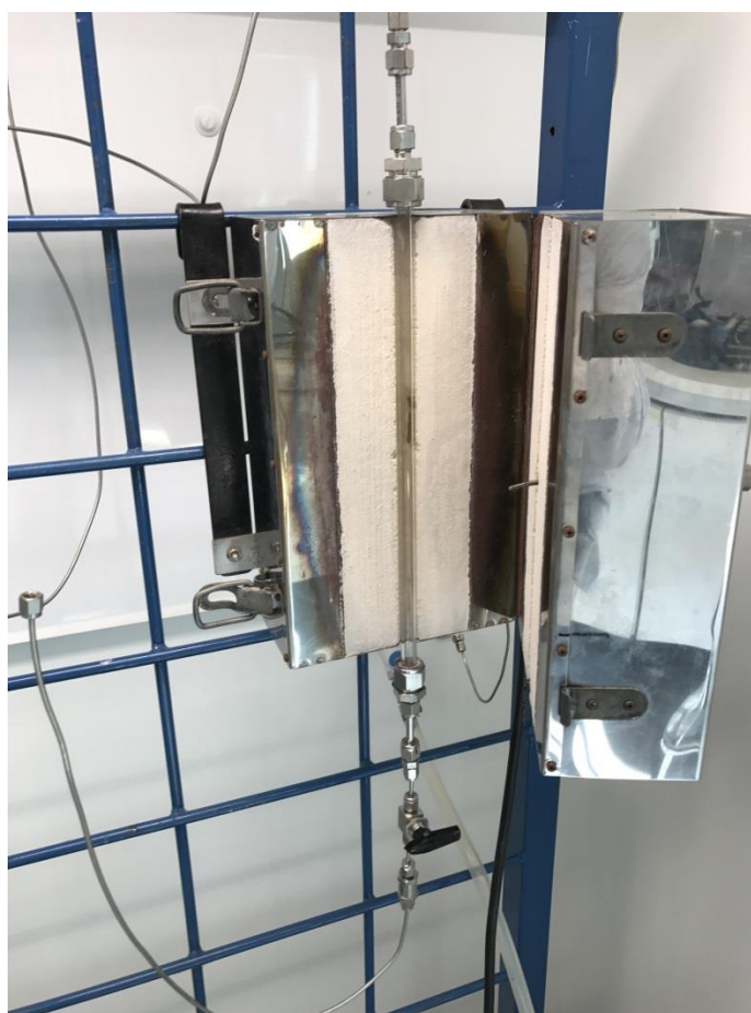
Figure 49 - Heated tubular contactor used for the catalyst activation.
