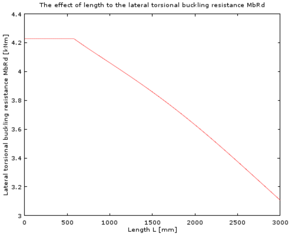
Figure 2.3. The effect of length of a beam to lateral torsional buckling resistance.
