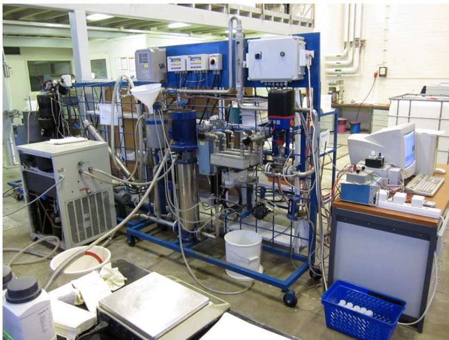
Figure 14. Cross-flow filtration setup with three cells.
