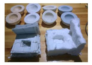
Figure 5.12: Sensor enclosures used in the test. Materials of the enclosures: In the bottom row, on the right SMG-128 wool and on the left WDS, in the upper row, from right to left, Super-1100E, Poromax26, JM23 and wood based enclosure halves
