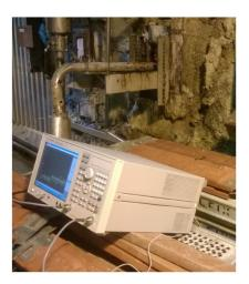
Figure 4.2: Vector network analyser (VNA) in measurements at kraft recovery boiler.
