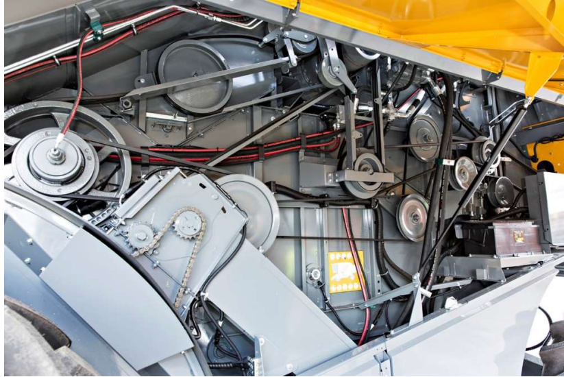
Figure 39. Pulleys and belts of Sampo-Rosenlew Comia C10 (Ahonen & Tuomi, 2016)
