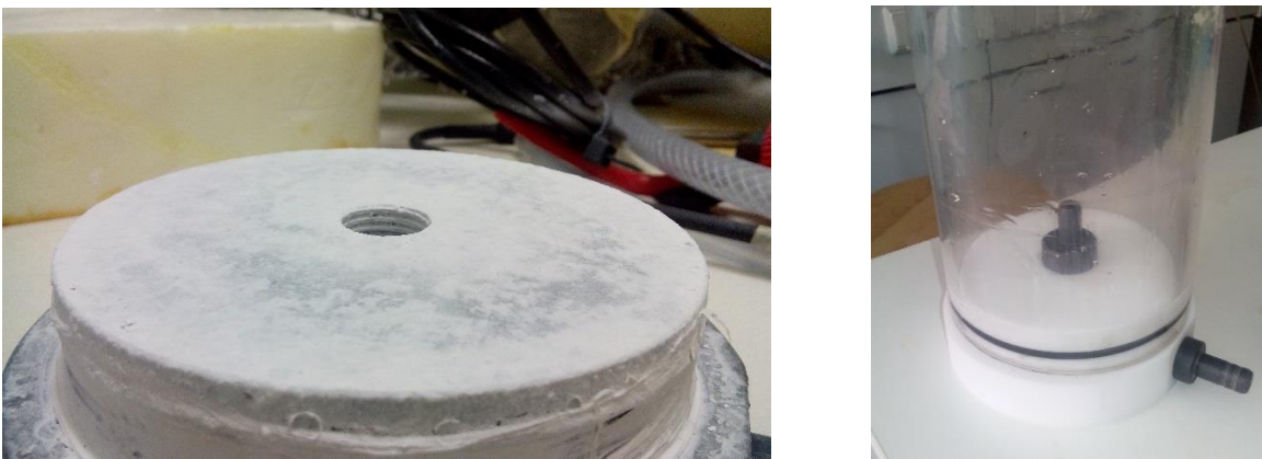
Figure 30. Teflon base plate with additional teflon spray coating
