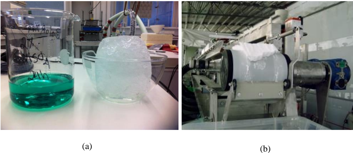
Figure 4. (a) Ice formation from nickel sulphate ( \text{NiSO}_4 ) solution in laboratory (b) Industrial output via freeze crystallization (FC technology process, 2017).
