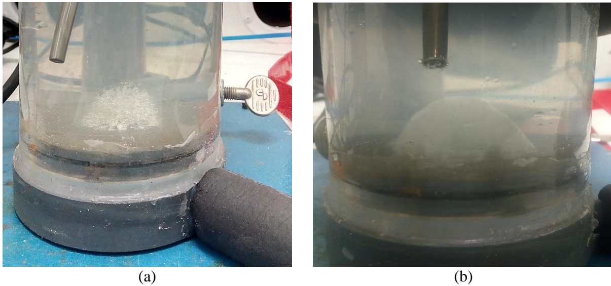
Figure 27. Ice formation at point of dispersion for (a) Pure water (b) Sodium sulphate solution
