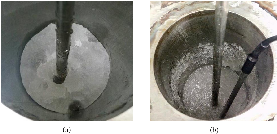
Figure 1. Different form of ice as obtained in the laboratory (a) Block of ice (b) Ice slurry
