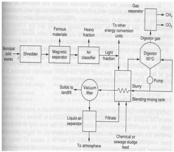
Figure 8: The low Solids anaerobic digestion process for the organic fraction of MSW flow diagram (Tchobanoglous and Kreith, 2002).
