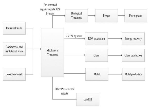
Figure 19: Mechanical treatment and biological process where RDF production for energy recovery, organic rejects for anaerobic digestion and other rejects for land fill.
