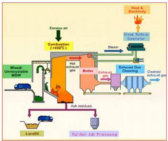
Figure 7: Incineration process (Moustakas and Loizidou, 2010).
