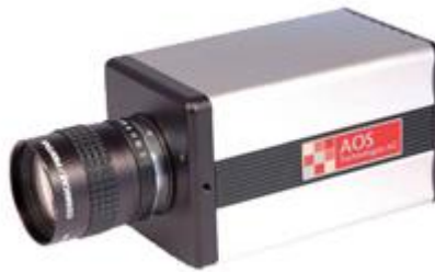
Figure 32. High-speed video camera X-Motion: color, resolution 1280x1024, pixel size 12 \mu\text{m} , shooting speed at full resolution 500 frame per second, speed shooting at reduced resolution 32000 frame per second, dynamic range 10 bit.
