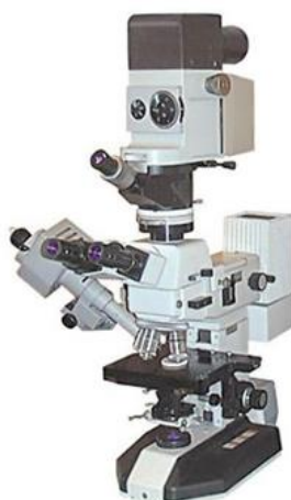
Figure 43. Microscope-spectrophotometer LOMO MSFU-K: range of spectral reflection 350-900 nm, range of diffuse reflection 380-760 nm, transmission range 350-900 nm, spectral range of luminescence 400-700 nm, magnification 50x-1000x, the minimum size of studied spot 1 \mu\text{m} .
