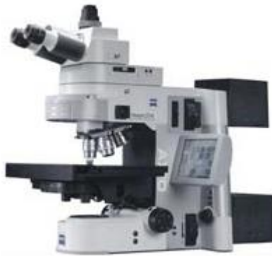
Figure 44. Universal microscope Axio Imager A1.m: magnification 100x-1600x, resolution (at least) 3800 lines per mm.
