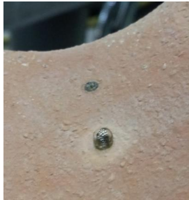
Figure 30. Plate of silicon dioxide ceramics with produced spheres above craters. Continuous-wave mode, power density 40 GW/m 2 , time of laser impact 1 second.
