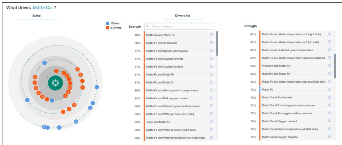
Figure 2.7. Determination of key drivers of copper content in matte by Watson Analytics spiral (Vanyukov Furnace 3 database)
