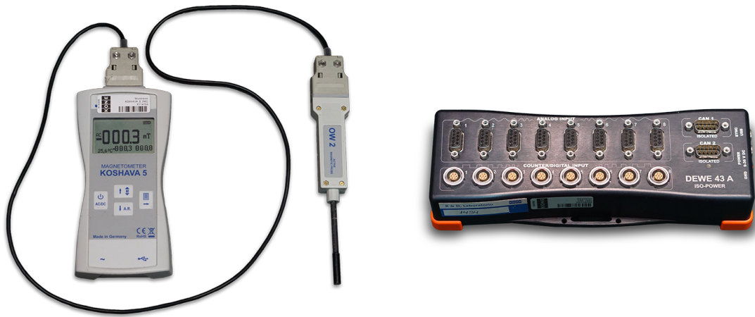
Figure 6.1. Instruments used in the measurements: a Wuntronic Koshava 5–magnetometer (left) and a Dewe43-A–unit (right)
