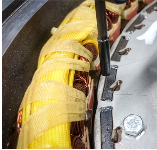
Figure 6.2. Measuring the PM edge flux from an IPMSM.
