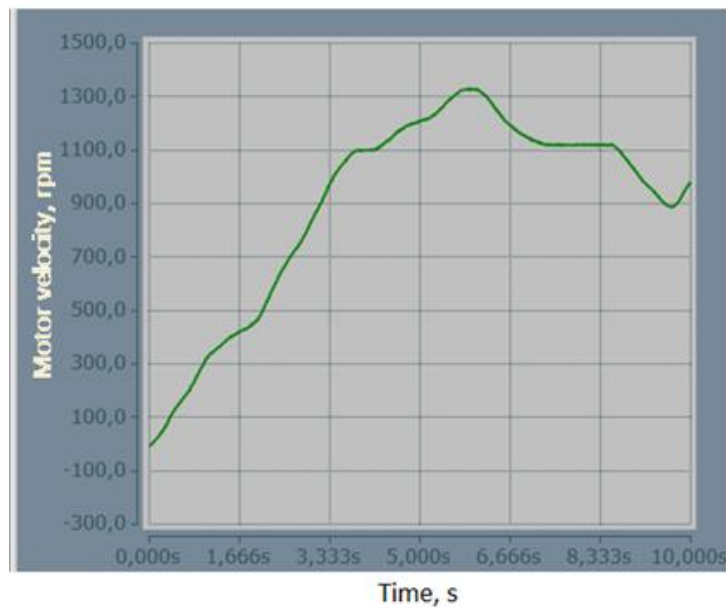
Figure 4.13. Servomotor rotational velocity scope in TwinCAT 3.
