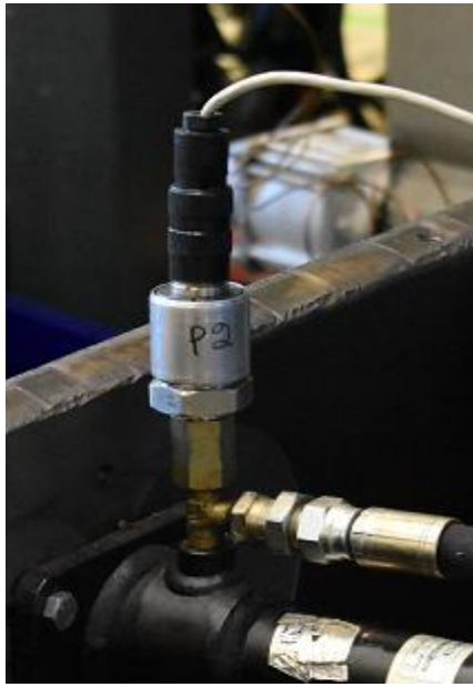
Figure 5.11. Pressure transducer utilized in hydraulic circuit (Bosch Rexroth AG Hydraulics 2005).
