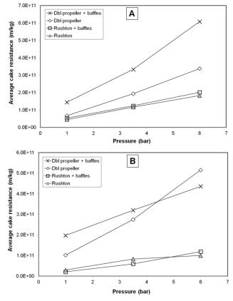
Fig. 6. Influence of baffles installed in the hydrolysis tank on average specific cake resistances at different filtration pressures. Rotation speed of the impellers (double propeller and Rushton turbine) 495 rpm, slurry solid contents 8 w-% (A) and 12 w-% (B).
