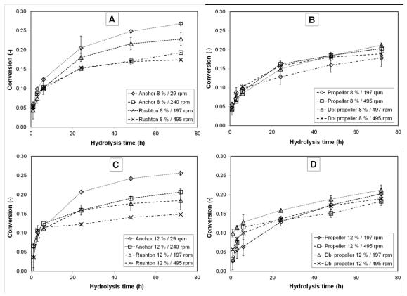
Fig. 3. Effect of rotation speed of the impeller and solids content of the slurry on the enzymatic conversion. Solids content of 8 % (A, B) and 12 % (C, D).
