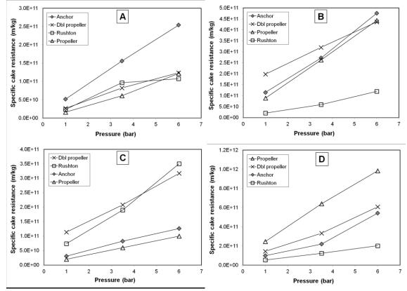
Fig. 5. Average specific cake resistances against applied filtration pressure. Slurry solids contents of 12 w-% (A, B) and 8 w-% (C, D). Slow (A, C) and fast (B, D) rotation speed of the impellers.
