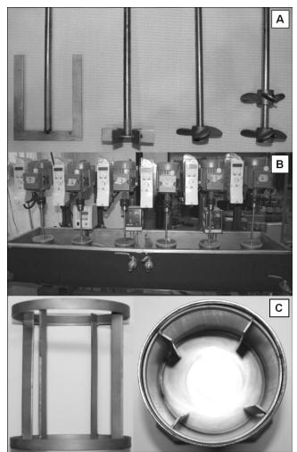
Fig. 1. The impellers left to right (A): Anchor, Rushton turbine, propeller, double propeller. The mixing device (B). The baffles and a mixing tank with the baffles (C).
