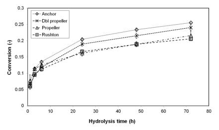
Fig. 2. Performance of the investigated impellers in enzymatic hydrolysis of the model biomass at 10 % solids content, medium rotation speed.
