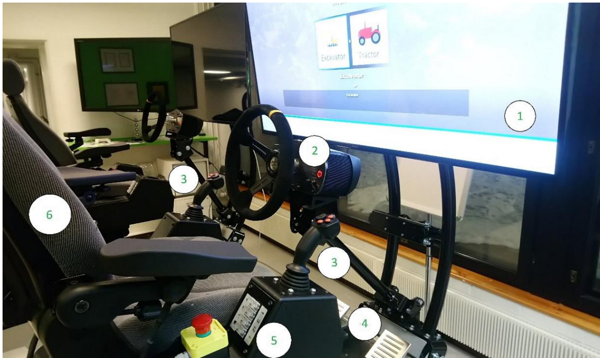
Figure 10: Structure of motion platform: 1-LED display, 2-steering wheel, 3-joysticks, 4-pedals, 5-control buttons, 6-seat.
