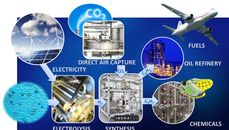
Figure 1: The main idea of the SOLETAIR Power-to-X process producing CO 2 neutral hydrocarbons with renewable electricity.
