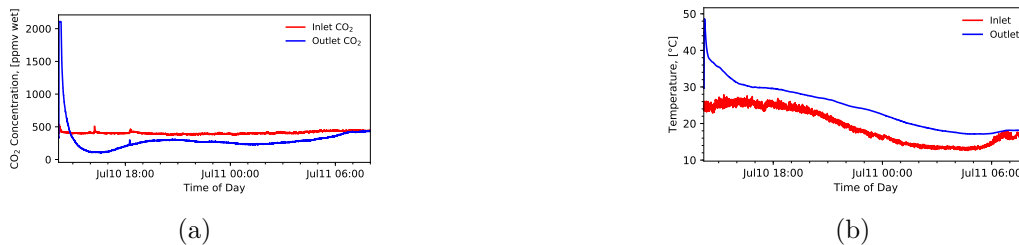
Figure 6: CO 2 and temperature at the inlet and outlet of beds 3 and 4. (a) CO 2 concentration. (b) Temperature.
