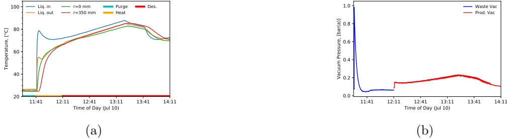
Figure 7: Key temperature and vacuum pressure measured for Bed 4 during the production phase. r is the radial distance from the center of the bed. The radius of a bed is 500 mm. (a) Temperature. (b) Vacuum pressure.
