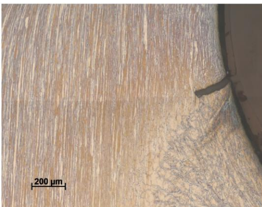
Fig. 20. A secondary crack that has grown in the coarse-grained ferrite phase of an X-joint in 2507.
