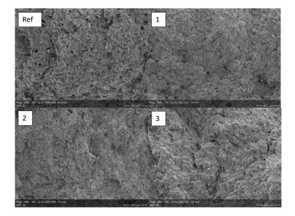
Figure 27: SEM-pictures of samples PLA with 40% BSKP (Ref), PLA+40% BSKP with 5% ELO (1), PLA+40% BSKP with 8% ELO (2) and PLA+40% BSKP with 12% ELO (3) with enlargement of 100.
