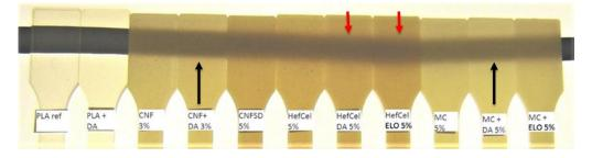
Figure 22: PLA composites with 3% or 5% CNF, 5% HefCel and 5% MC with and without DA and ELO. Red arrows showing the effect of DA and ELO in PLA-HefCel composites. Black arrows shows the effect of DA on 3% CNF and MC PLA-composites.
