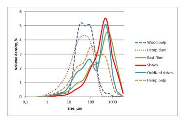
Figure 20: Particle size distributions of fibre materials removed from injection moulded PLA-fibre composites from work described in Paper III. Wood pulp is softwood cellulose.
