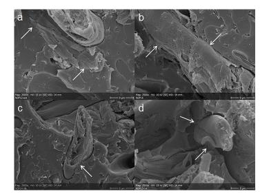
Figure 29: SEM-pictures of samples PLA+30% BSKP with 1% moisture (a), 3% moisture (b), 16% moisture (c) and 25% moisture (d) in fibre at the beginning of compounding. Pictures with enlargement of 2500. The arrows indicate fibre-polymer interfaces.
