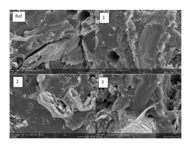
Figure 28: SEM-pictures of samples PLA with 40% BSKP (Ref), PLA+40% BSKP with 5% ELO (1), PLA+40% BSKP with 8% ELO (2) and PLA+40% BSKP with 12% ELO (3) with enlargement of 2500.
