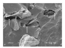
Figure 30: SEM-picture of PLA-birch pulp (20%) composite with the enlargement of 2500. The arrows indicate the gap in polymer-fibre interface.
