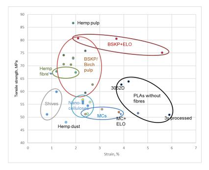
Figure 17: Tensile strength versus strain distribution for all the results in five papers. The circles around results are grouping the composites with similar fibre types and also indicated with the same colour as text.
