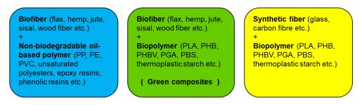
Figure 2: Classification of biocomposites according to constituents (Mitra 2014).
