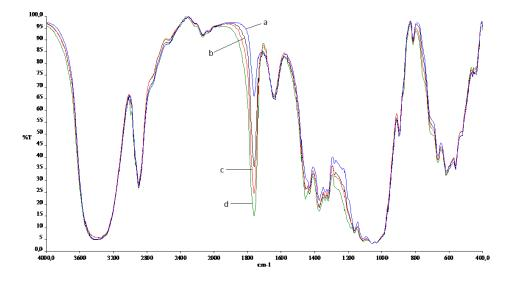
Figure 31: FTIR-spectra of cellulose samples after dissolving out the loose PLA. Spectrum a) is PLA with 40% BSKP (Ref), b) PLA+40% BSKP with 5% ELO, c) is PLA+40% BSKP with 8% ELO (2) and d) is PLA+40% BSKP with 12% ELO.
