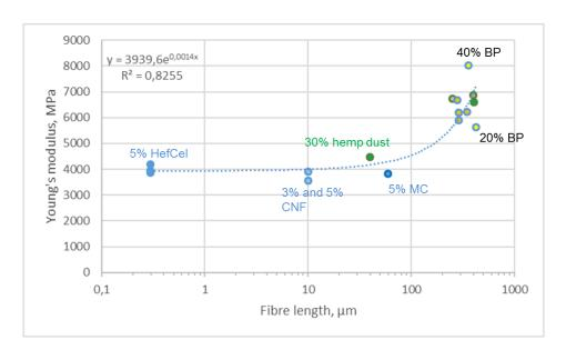
Figure 21: Fibre length in correlation to tensile modulus (Young's modulus). Fibre lengths are after compounding and injection moulding except with CNF, HefCel) and MC those are values before processing. The probability  $R^2$  for exponential fit is 0.8255.
