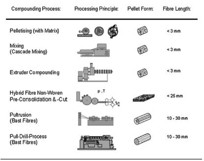
Figure 12: Compounding methods for injection moulding of natural fibre reinforced thermoplastic composite granules (Faruk et al. 2012).
