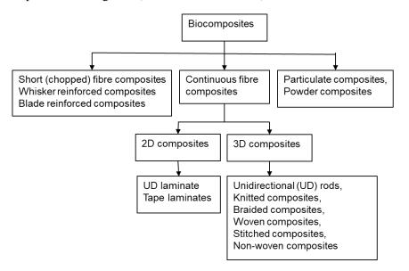
Figure 1: Classification of biocomposites according to architectural structure (Ramakrisna et al. 2004).
