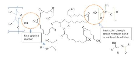
Figure 32: Suggested reaction schema for cellulose fibre PLA coupling with epoxidised linseed oil (ELO).
