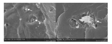
Figure 26: SEM-pictures of 5% HefCel- (left) and MC-containing (right) PLA composites with ELO as additive. The arrows indicate the interface between fibre and polymer.
