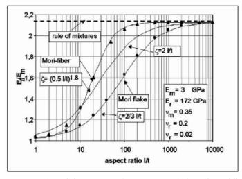
Figure 13: Plot of the computed Young's modulus of a unidirectional composite filled with flakes or fibres of different aspect ratios using the Tsai– Halpin and the Mori– Tanaka model. In both cases, a stronger reinforcing action of the fibres compared to platelets can be predicted (Gacitua et al. 2005)
