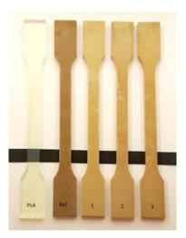
Figure 23: Injection moulded test samples from left to right PLA, PLA with 40% BSKP (Ref), PLA+40% BSKP with 5% ELO (1), PLA+40% BSKP with 8% ELO (2) and PLA+40% BSKP with 12% ELO (3).
