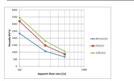
Figure 24: Apparent melt viscosity at 190°C for 40% BSKP fibre-containing PLA samples.
