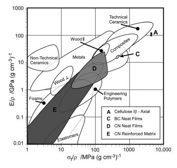
Figure 9: Ashby plot of specific modulus  $(E/\rho)$  versus specific strength  $(\sigma/\rho)$ . Regions of crystalline cellulose I $\beta$  (A), BC neat films (C), neat films of either CNC, t-CNC, MFC, and NFC (D), and NC-reinforced matrix composites (less than 30 wt% NC) (E). (Moon et al. 2011)
