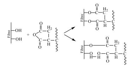
Figure 10. The reactions between cellulose fibre and maleic grafted polymer.
