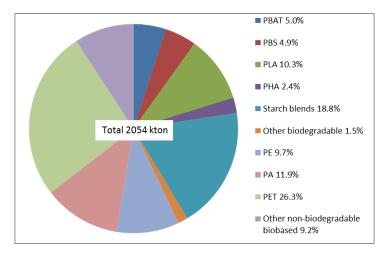
Figure 5: Global production capacities of bioplastics in 2017 by material type (without PUR; reproduced data from European Bioplastics 2018).
