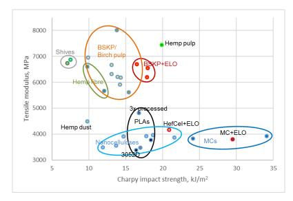
Figure 18: Tensile modulus versus Charpy impact strength distribution for all the results in five papers. The circles around results group the composites with similar fibre types and also indicated with the same colour as text.
