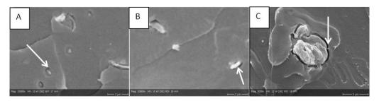
Figure 25: SEM-pictures of 5% CNF (A), HefCel (B) and MC (C) containing PLA composites without additives. The arrows indicate the gap between fibre and PLA.
