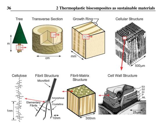
Figure 8: Hierarchial structure of wood from tree to cellulose (Moon et al. 2011)
