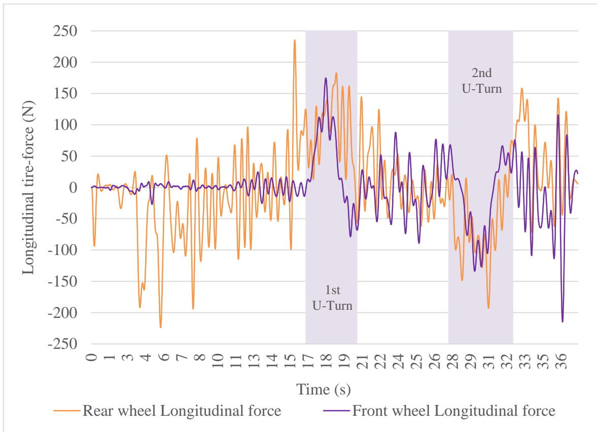
Figure 25. Plot of the front and rear wheel longitudinal tire-forces over time.
