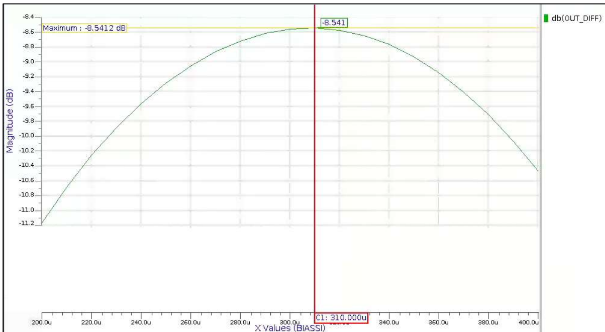
Figure 5.5. The magnitude of the differential output voltage as a function of the bias current to determine the bias current with which the gain is at its highest.
