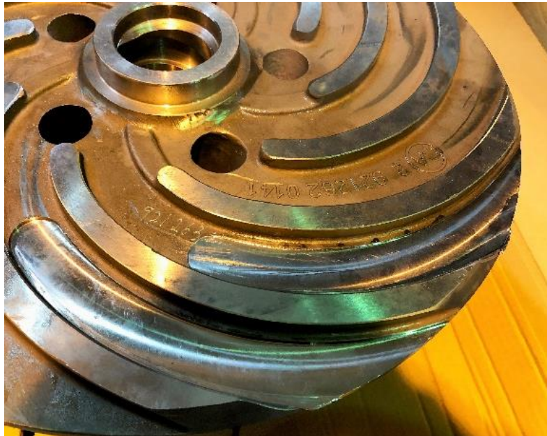
Figure 27. Impeller after correction by CNC-milling. Achieved surface quality meets the requirements.
