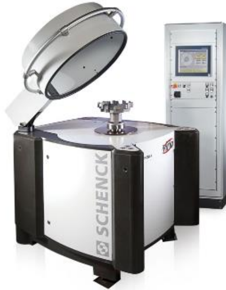
Figure 22. Recommended vertical balancing machine for unbalance measurement (VIRIO).
